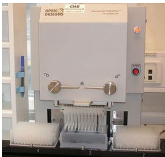
Figure 8. Automated liquid handling system used for 96-tips sample preparation.
