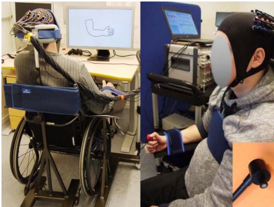
Fig. 1. fNIRS experimental set-up. Foam-covered pads were used to apply the specially designed adult optical fibers firmly but comfortably to the subjects' heads. Subjects were seated with the forearm supported on an adjustable table, and the wrist strapped. Due to very limited or complete loss of trunk stability in patients, a specially designed and portable neck rest was constructed that the subjects were strapped towards, with the aim of minimizing movement of the torso. A small cube was attached to the index finger to keep the thumb stabilized and somewhat elevated in relation to the index finger. Permission was granted by the patient.
