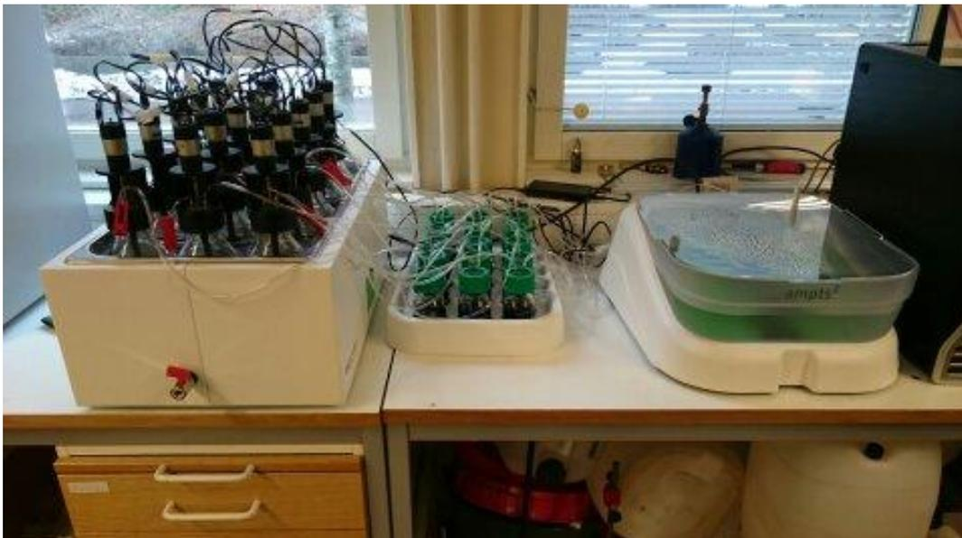
**Figure 3** The equipment AMPTS2. The digestion chamber is to the left, in the middle is the CO<sub>2</sub>-fixation unit and to the right is where the produced gas is measured.
