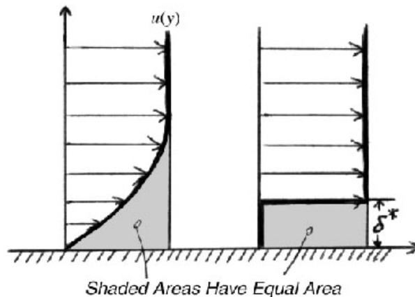
Figure 3: Velocity distribution for a real fluid and the displacement thickness. [c]
