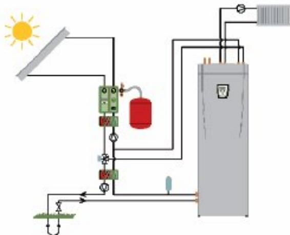
Figure 1: Image of a heat pump and solar collector system. [a]
