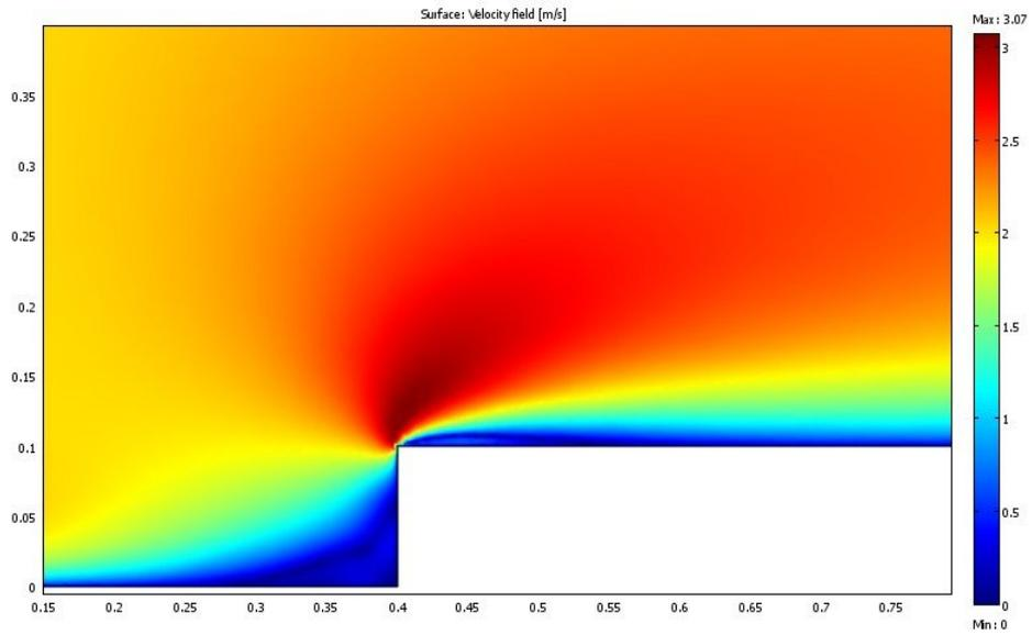
**Figure 9:** Image of the velocity field around the edge of the solar collector. The incoming wind speed is 2 m/s. The edge creates a wake.
