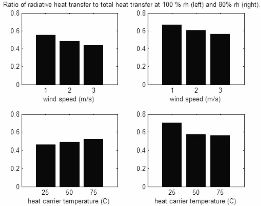
**Figure 7: Ratio of the radiative heat transfer to the total heat transfer at 100 % and 80 % relative humidity.**
