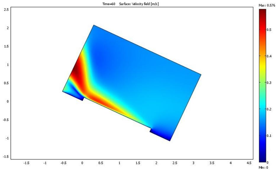
**Figure 11: Image of the air flow around the solar collector on the roof, due to natural convection, after 60 s simulation. See colored bar to the right for wind speed. The temperature of the plate is 50°C and the air temperature is 10°C.**
