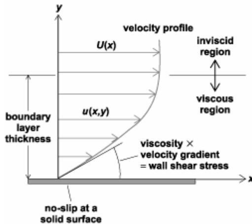
Figure 2: Velocity profile of the boundary layer. [b]
