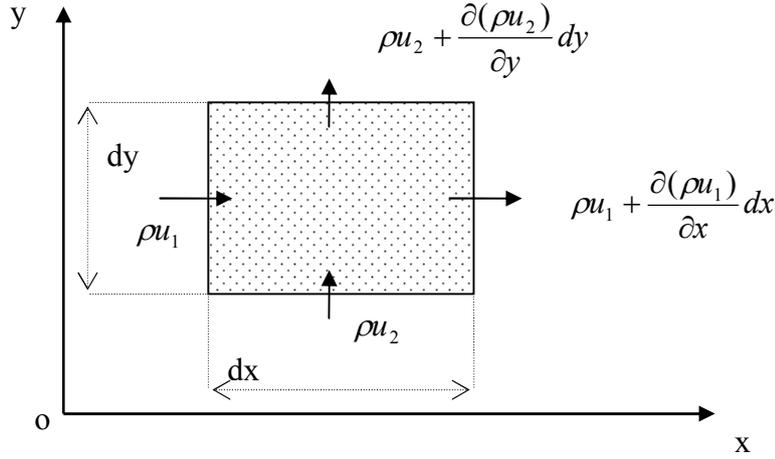
By taking the difference between the inflow and the outflow in the x and y directions, the fluid mass stored in the respective directions per unit time can be obtained as  $-\frac{\partial(\rho u_1)}{\partial x} b dx dy$  and  $-\frac{\partial(\rho u_2)}{\partial y} b dx dy$  respectively. The initial mass of the fluid element is  $\rho b dx dy$ , and this should increase by  $\frac{\partial(\rho b dx dy)}{\partial t}$ . [8b]
