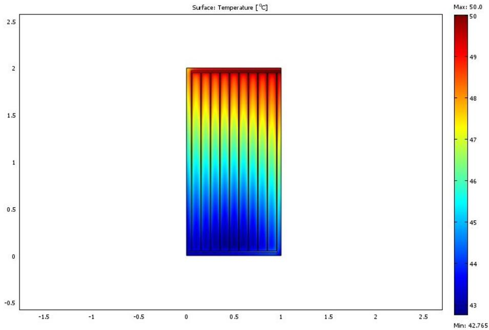
**Figure 10:** Image of surface temperature of the solar collector. The air temperature is 15°C, the ambient temperature 15°C, the inlet fluid temperature 50°C, the air velocity 2 m/s and the fluid flow rate 2 l/min. The temperature of the plate is lower between the tubes than by the tubes.
