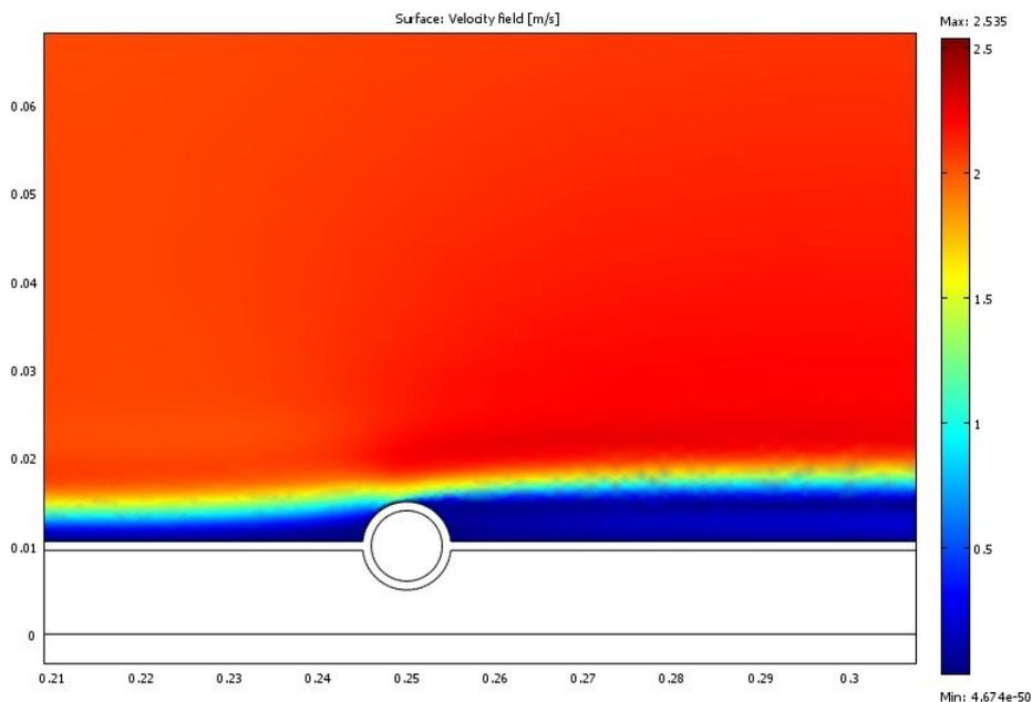
**Figure 8: Image of the wake caused by the tubes.**
