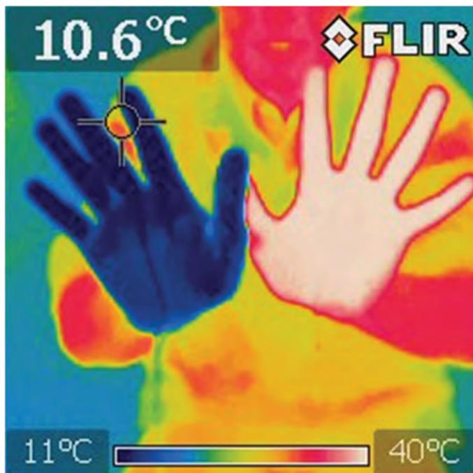
**Figure 1.** IR image captured with a FLIR i3 camera following submerging one's hands in cold (left) and warm (right) water.
