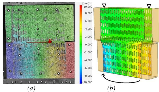
**Figure 3:** Punched metal plate connection loaded in twist by 1.73 kNm with colour plot for the out-of-plane displacements. (a) Illustration of Aramis-measured displacements. (b) Simulated twist deformations of tested connection specimen.
