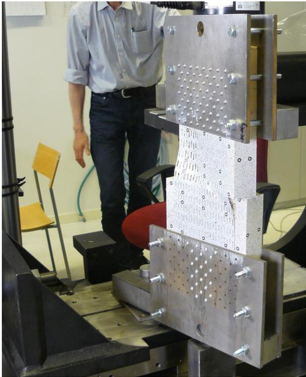
**Figure 2:** Two timber boards connected by punched metal plate fasteners from both sides. Ends of the boards are fixed to the MTS biaxial machine with a twist test setup.
