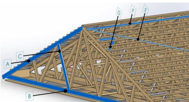
**Figure 1:** Pitched timber roof structure with semi-rigid bracing system of wood: A-top chord, B-bottom chord, C-diagonal, D-bracing truss, E-wind brace, F-roof battens.
