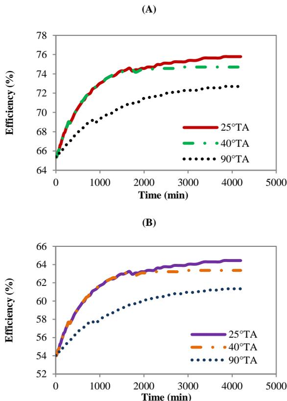
**Fig. 5:** Influence of Varied Throat Angle on Efficiency of Gasification: (A) Torrefied Bagasse Gasification from this Study; (B) Untorrefied Bagasse Gasification from A Previous Study [4].
