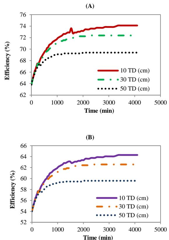
**Fig. 6:** Influence of Varied Throat Diameter on Gasification Efficiency: (A) Torrefied Bagasse Gasification from this Study; (B) Untorrefied Bagasse Gasification from A Previous Study [4].
