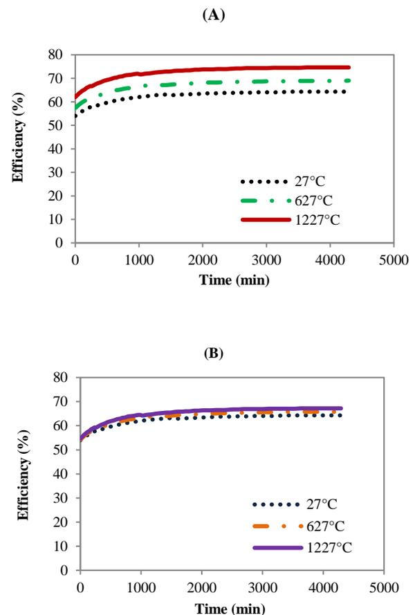
**Fig. 4:** Influence of Varied Temperature of Input Air on the Efficiency of Gasification: (A) Torrefied Bagasse Gasification from this Study; (B) Untorrefied Bagasse Gasification from A Previous Study [4].
