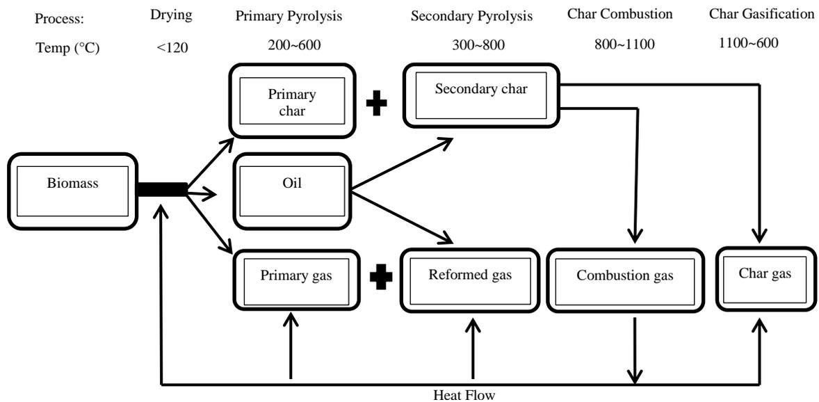
Fig. 1: Heat and Mass Flows in A Gasification Process. Adapted From [6].
