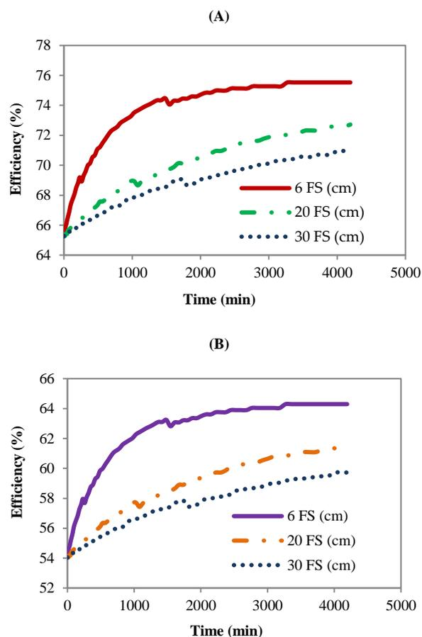
Fig. 2: Influence of Varied Feed Size on the Efficiency of Gasification: (A) Torrefied Bagasse Gasification from This Study; (B) Untorried Bagasse Gasification from A Previous Study [4].
