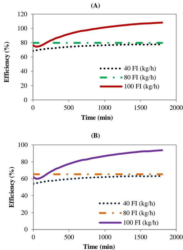
**Fig. 3:** Influence of Varied Feed Input on Gasification Efficiency: (A) Torrefied Bagasse Gasification from This Study; (B) Untorrefied Bagasse Gasification from A Previous Study [4].
