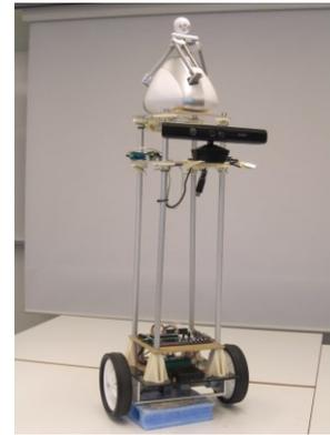
Figure 3. The multipurpose human-friendly assistive robot vehicle (*KFriend*) developed at Karlstad University
