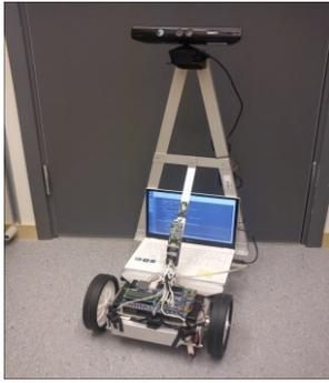
Figure 1. Human-friendly robot vehicle for carrying-medical tools (*iCAR*) developed at Karlstad University.
