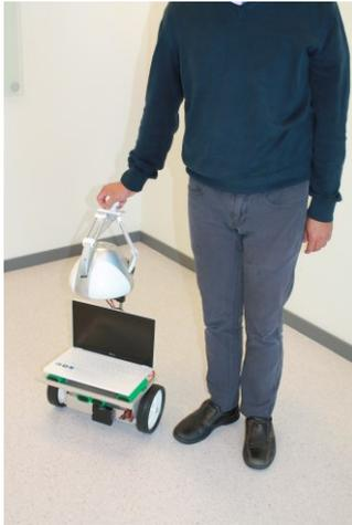
Figure 2. Human-friendly walking assisting robot vehicle (*hWALK*) developed at Karlstad University.
