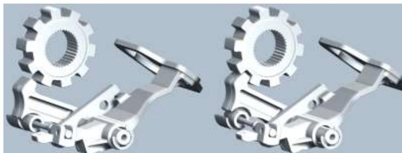
Figure 3. To the left, PLM disengaged. To the right, PLM engaged.
