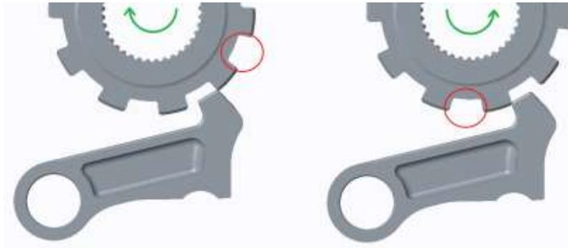
Figure 2. Schematic picture on rollback on the PLM, both rollaway when park up the slope and down the slope.
