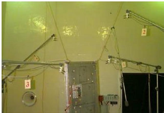
Figure 4-10. Acoustic test with a plate strung up with a component attached [26]
