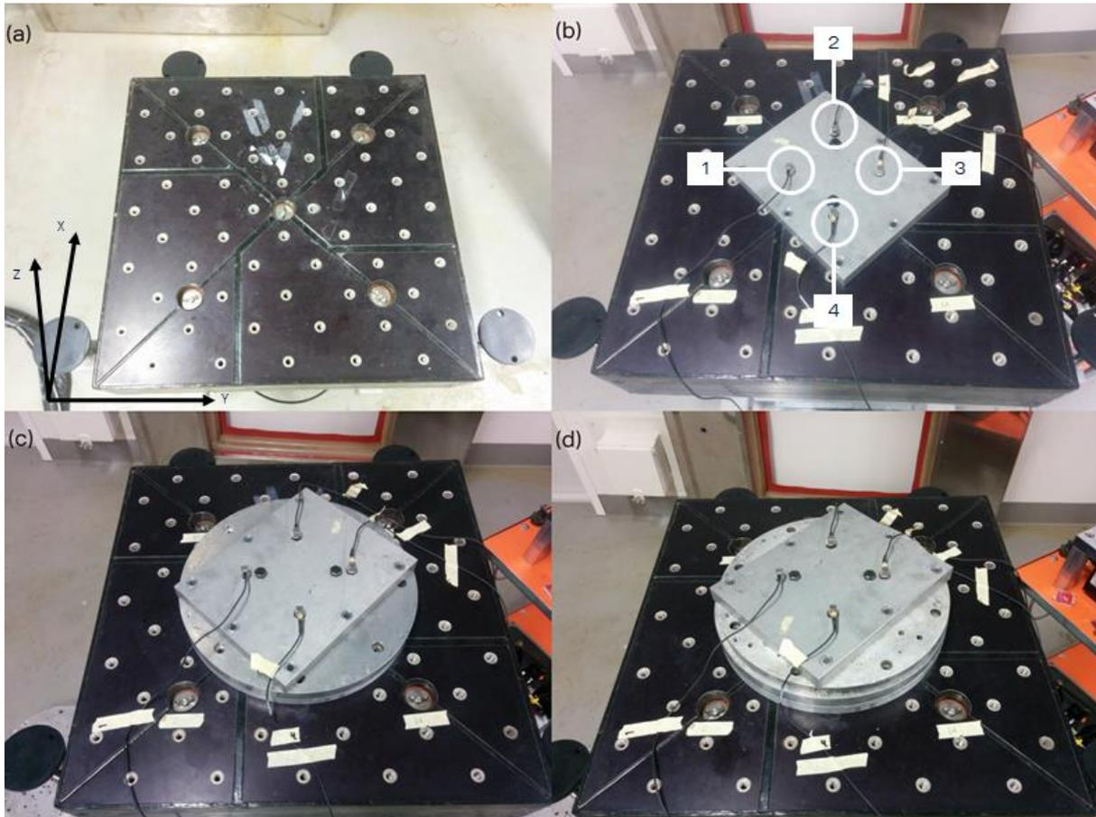
Figure 5-5. RS system for measuring the difference in response with different amount of mass (aluminium plates) (a) 1<sup>st</sup> test Empty table, (b) 2<sup>nd</sup> response test illustrating the position of the 4 accelerometers and their position, (c) 3<sup>rd</sup> response test, (d) 4<sup>th</sup> response test.
